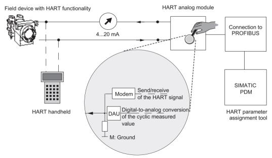
Figure 4-2 System environment for the use of HART
